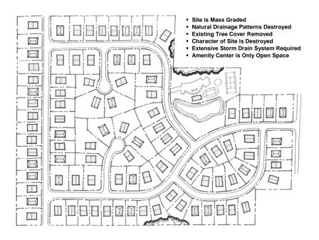
Figure 48: Residential Subdivision - Conventional Design (Source: Georgia Stormwater Manual, 2001)
