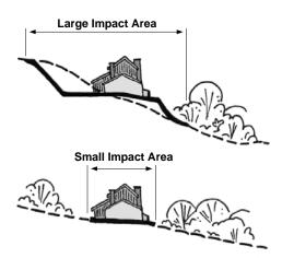
Figure 7: Grading that Creates Large Construction "Pads" Impacts more Land than Contoured Grading on Smaller Areas at Flatter Slopes (Source: MPCA, 1989)
