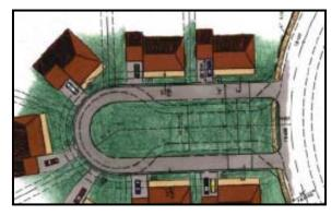
Figure 22: Loop Road Option (Source: Center for Watershed Protection, 2005)
