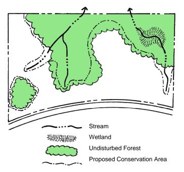
Preservation areas should then be incorporated into site development plans and clearly marked on all construction and grading plans to ensure that construction activities are kept out of these areas and that native vegetation is kept in an undisturbed state. The boundaries of each conservation area should be mapped by carefully determining the limit which should not be crossed by construction activity.
