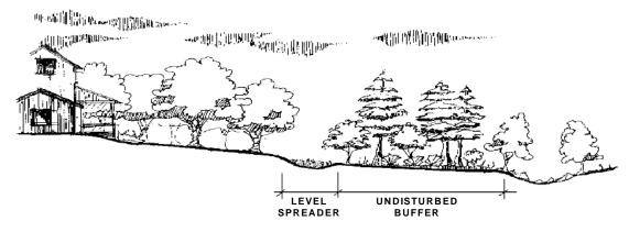
Figure 30: Use of a Level Spreader with a Riparian Buffer (Source: Georgia Stormwater Manual, 2001)
