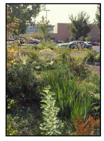
Figure 32: Use of a Vegetated Filter Strip (Source: MA EOEA, 2005)
