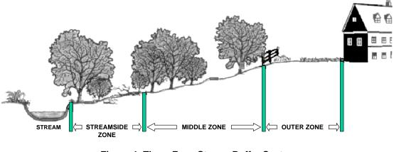
Figure 4: Three-Zone Stream Buffer System (Source: Adapted from Schueler, 1995)
