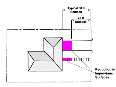
Figure 18: Reduced Driveway and Walkway Lengths by Using Reduced Setbacks (Adapted from: MPCA, 1989)
