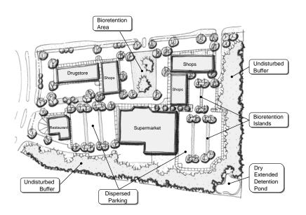
Figure 51: Commercial Development - Better Site Design (Source: Georgia Stormwater Manual, 2001)
