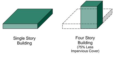
Figure 24: Reduction of Impervious Cover by Building Up Rather than Out (Source: Georgia Stormwater Manual, 2001)
