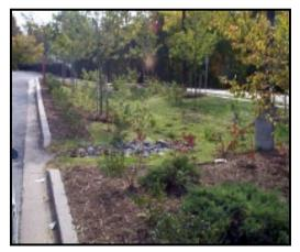
Figure 35: Example of a Bioretention Facility in a Parking Lot Island
