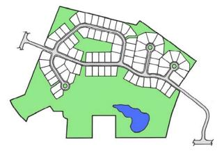
Figure 11: Example of an Open Space or "Cluster" Subdivision Example (Source: Georgia Stormwater Manual, 2001)
