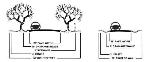
Figure 15: Potential Design Options for Narrower Roadway Widths (Source: Georgia Stormwater Manual, 2001)
