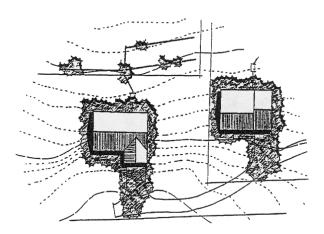
Figure 5: Establishing Limits of Clearing (Source: DDNREC, 1997)
