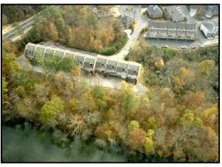
Figure 6: Example of Site Foot-Printing (Source: Georgia Stormwater Manual, 2001)
